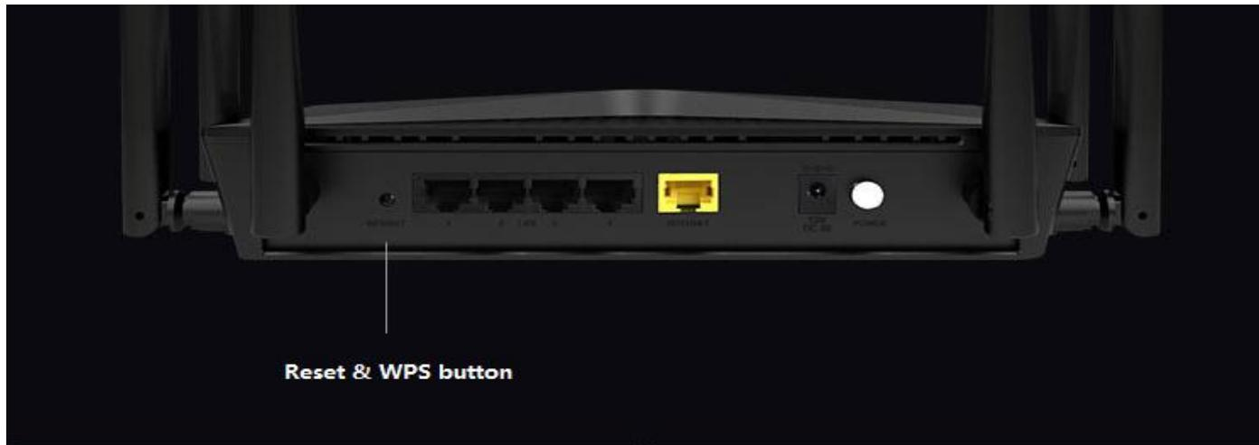
**Step 2** - Within 2 minutes, press the WPS button on your wireless device (or launch the software utility and start the WPS process).
